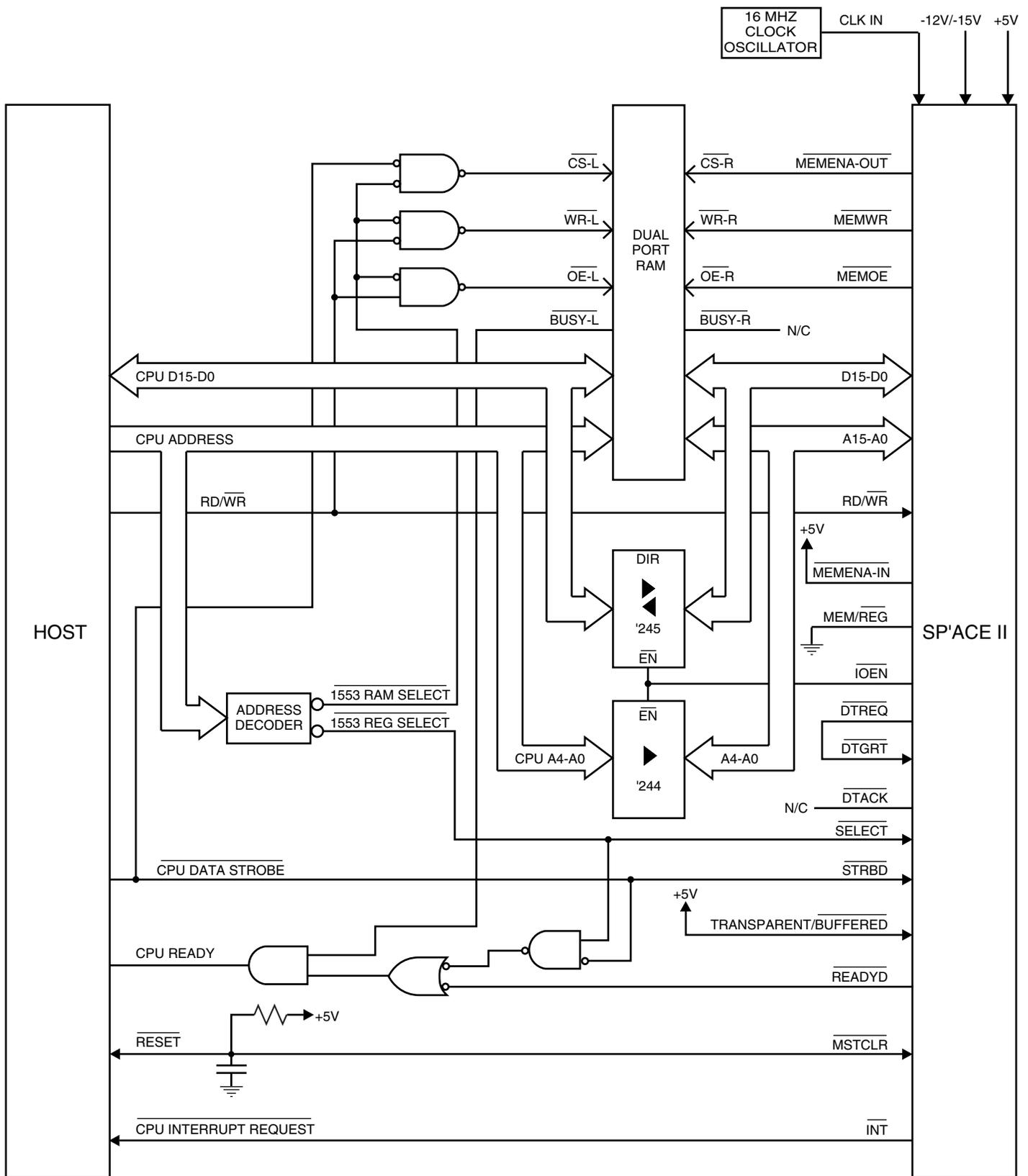
FIGURE 11. 16-BIT TRANSPARENT MODE USING DUAL PORT RAM
