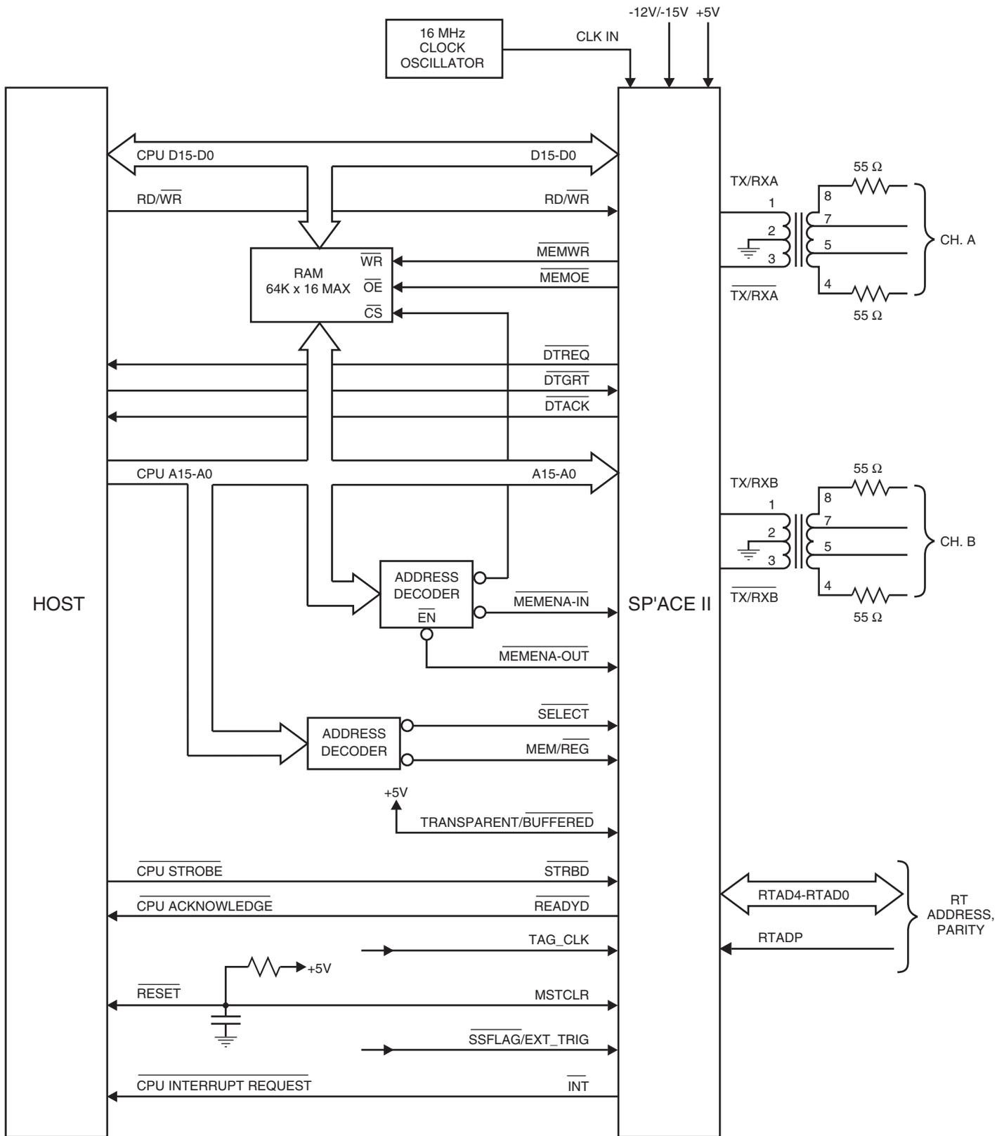
**FIGURE 12. 16-BIT DIRECT MEMORY ACCESS (DMA) MODE**
