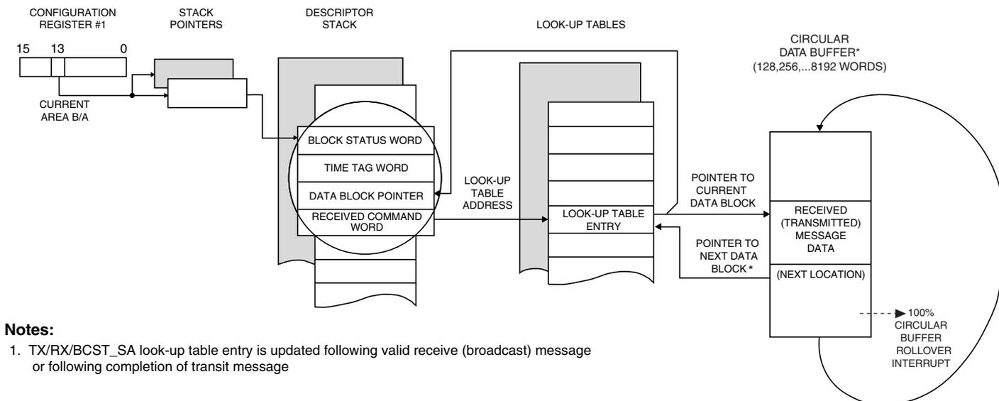
**FIGURE 6. RT MEMORY MANAGEMENT: CIRCULAR BUFFER MODE**
