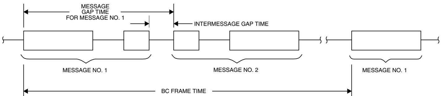
**FIGURE 2. BC MESSAGE GAP AND FRAME TIMING**
