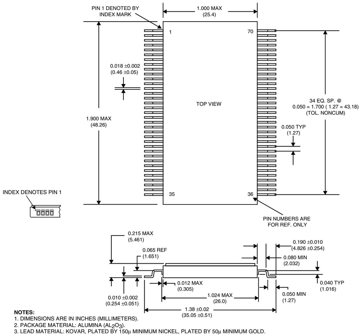
**FIGURE 21. BU-63825GX, 70-PIN GULL LEAD CERAMIC MECHANICAL OUTLINE**
