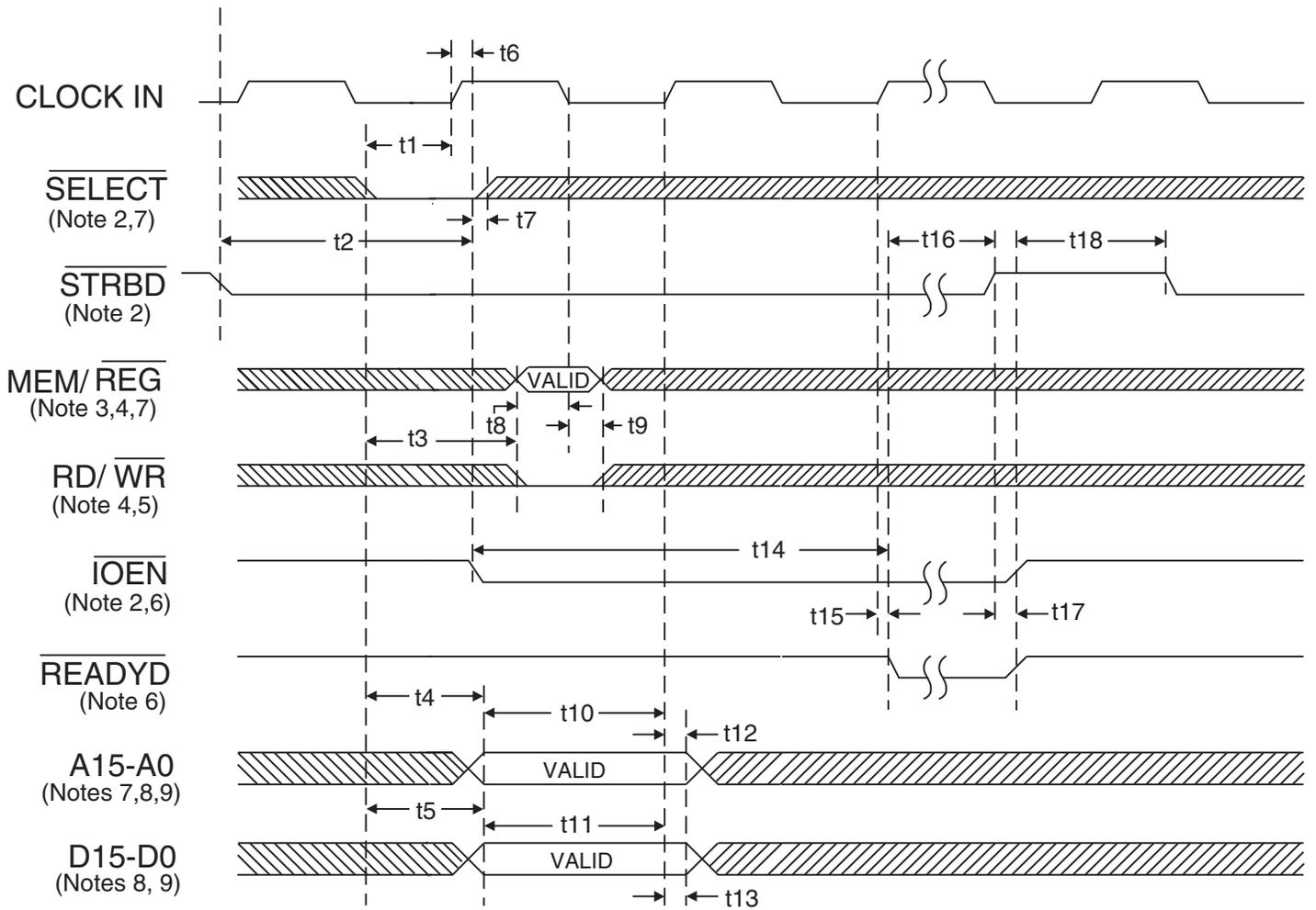
**FIGURE 17. CPU WRITING RAM (SHOWN FOR 16-BIT, BUFFERED, NONZERO WAIT MODE, UNCONTENDED ACCESS)**
