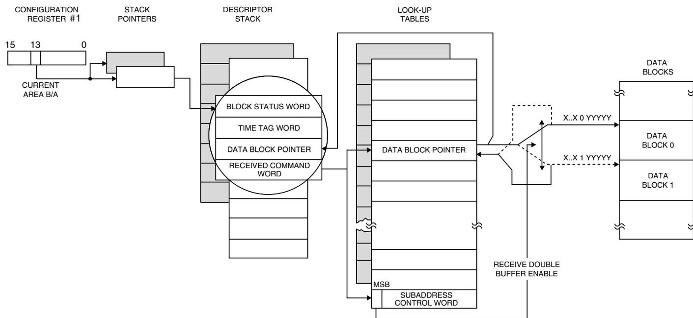
**FIGURE 7. RT MEMORY MANAGEMENT: SUBADDRESS DOUBLE BUFFERING MODE**
