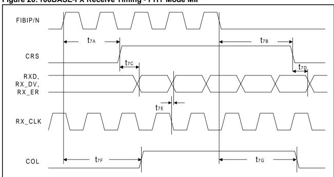
Figure 20: 100BASE-FX Receive Timing - PHY Mode MII
