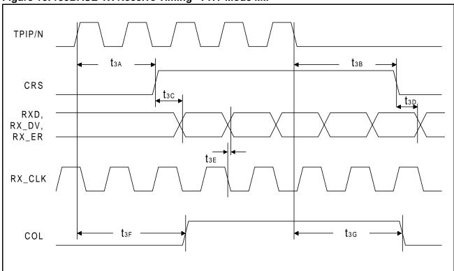
Figure 16: 100BASE-TX Receive Timing - PHY Mode MII
