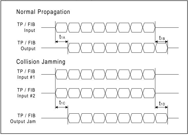
Table 21: 100 Mbps Port-to-Port Delay Timing Parameters
