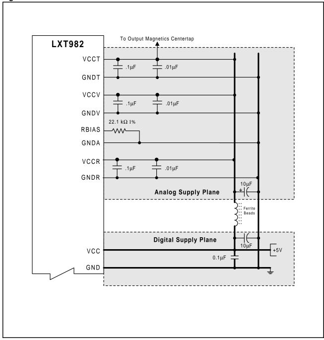
Figure 9: Power and Ground Connections
