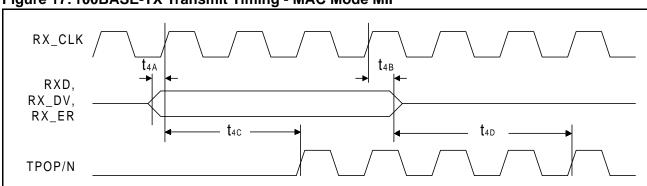
Figure 17: 100BASE-TX Transmit Timing - MAC Mode MII
