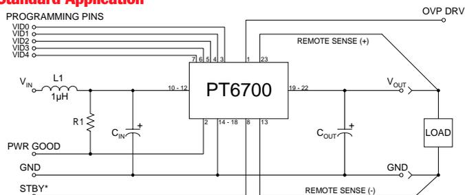
$C_{in}$  = Required 1000 $\mu$ F electrolytic
