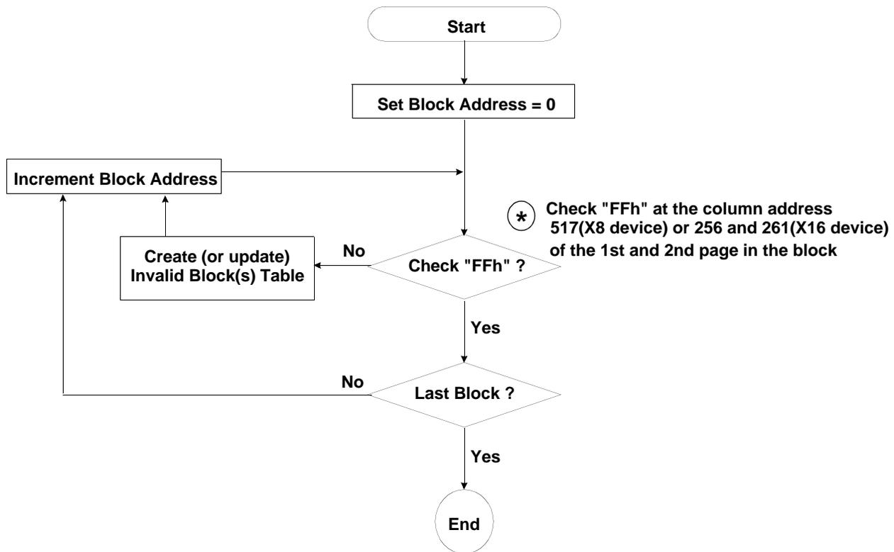
Figure 11. Flow chart to create invalid block table.
