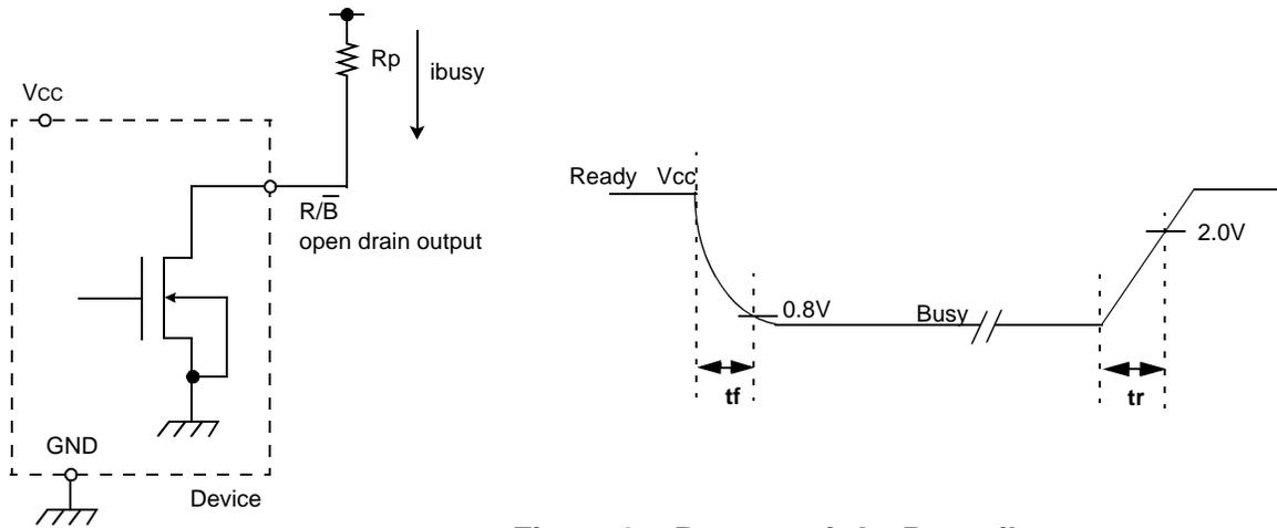
**Figure 9. Rp vs tr ,tf & Rp vs ibusy**
