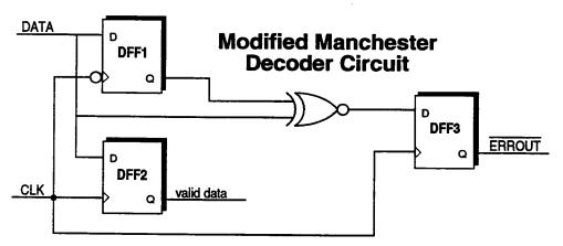
RULE: Must have different values on the rising and falling edges when sampling the falling edge first. Valid data is read on the rising edge of CLK.
