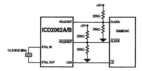
The ICD2062A/B may drive the CLOCK inputs of up to four RAMDACs, if they are located physically adjacent to each other. In this case, only 2 sets of termination resistors should be used, and these should be located nearest the farthest RAMDAC from the ICD2062A/B.
