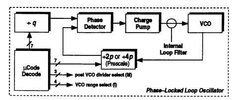
Each oscillator block is a classical phase-locked loop connected as shown above. The external input frequency f(REF) goes into a divide-by-n block. The resultant signal becomes the reference frequency for the phase-locked loop circuitry.
