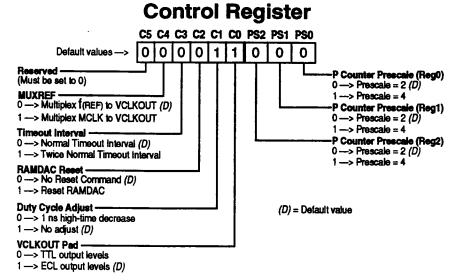
MUXREF — This control bit determines which clock is multiplexed to the VCLKOUT output during frequency changes. While the VCLK VCO changes to a different frequency, a known clock is multiplexed to the output. The default is to multiplex the f(REF) reference frequency, but some graphic controllers cannot run as slow as f(REF). This bit, when set, allows the MCLK to be used as an alternative frequency.
