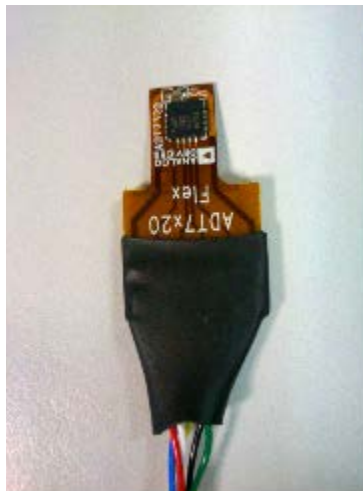
Figure 3. ADT7320FBZ Evaluation Board—External Board
