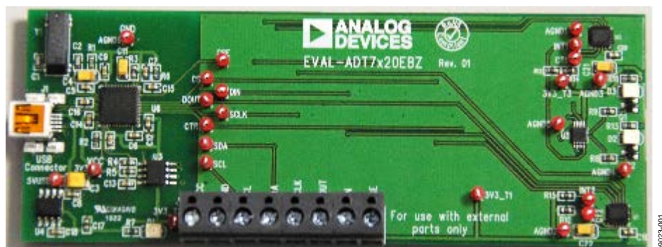
Figure 1. ADT7x20 Evaluation Board—Main Board
