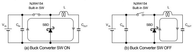
Fig. 5. Current Loop at Buck Converter
