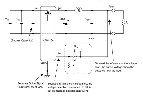
Fig. 6. Board Layout at Buck Converter
