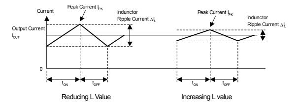
Fig. 4. Inductor Current State Transition (Continuous Conduction Mode)
