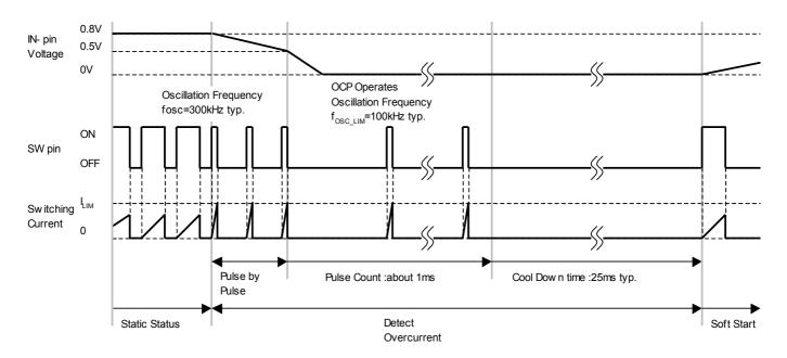
Fig. 2. Timing Chart at Over Current Detection
