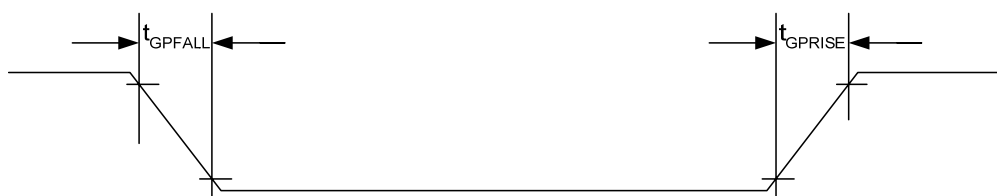
Figure 12: Output Rise/Fall Time
