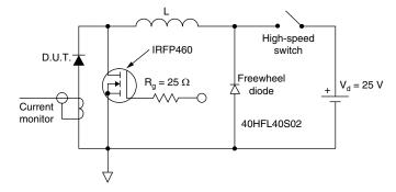
Fig. 7 - Unclamped Inductive Test Circuit
