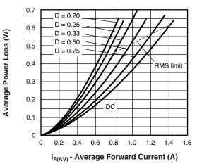
Fig. 5 - Forward Power Loss Characteristics (Per Leg)
