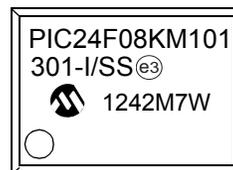
28-Lead SSOP (5.30 mm)
