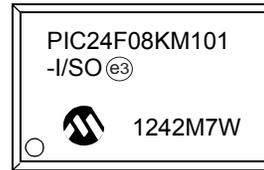
28-Lead SOIC (7.50 mm)
