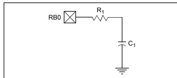
A timer can be used to measure the charge time and discharge time of the capacitor. The charge time can then be adjusted to provide the desired delay in Sleep. This technique compensates for the affects of temperature, voltage and component accuracy. The peripheral can also be configured as a simple, programmable Low-Voltage Detect (LVD) or temperature sensor.
