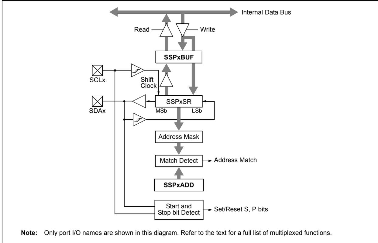
**FIGURE 14-4: MSSPx BLOCK DIAGRAM (I<sup>2</sup>C™ MASTER MODE)**
