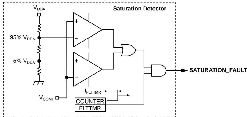
Figure 10. Saturation Detector
