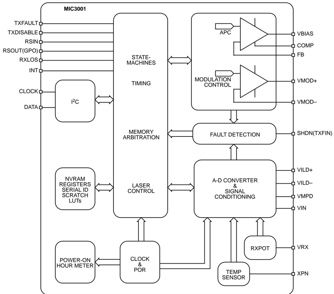
Figure 1. MIC3001 Block Diagram
