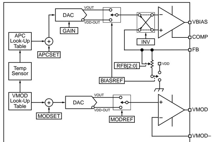
**Figure 4. MIC3001 APC and Modulation Control Block Diagram**
