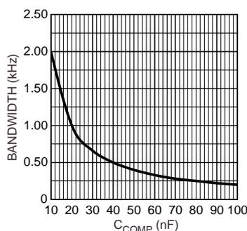
Figure 29. Open Loop Unity-Gain Bandwidth vs.  $C_{COMP}$
