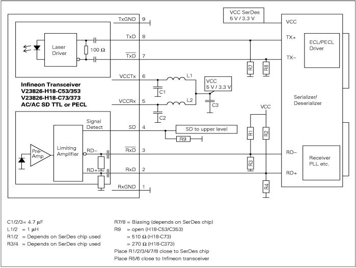
Values of R1/2/3/4 may vary as long as proper 50  $\Omega$  termination to  $V_{EE}$  or 100  $\Omega$  differential is provided. The power supply filtering is required for good EMI performance. Use short tracks from the inductor L1/L2 to the module  $V_{CC}Rx\mathcal{N}_{CC}Tx$ .
