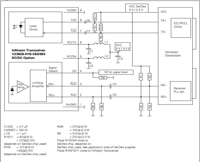
The following Application Notes assume Fiber Optic Transceivers using 5 V power supply and SerDes Chips using 3.3 V power supply. It also assumes no self biasing at the receiver data inputs (RD+/RD-) of the SerDes chip (Refer to the manufacturer data sheet for other applications). 3.3 V-Transceivers can be directly connected to SerDes-Chips using standard PECL Termination network.
