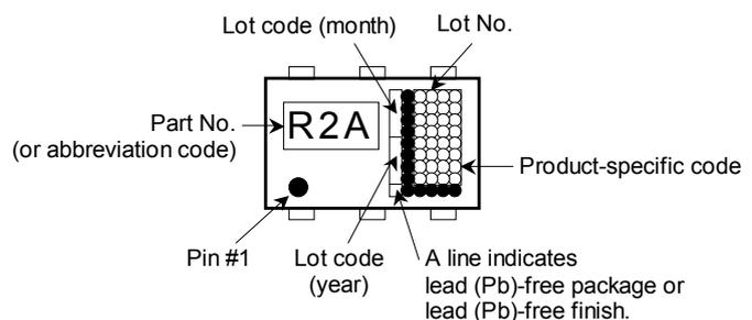
The round black marking "●" located on the lower left of the parts number marking "R2A" indicates terminal No. 1.
