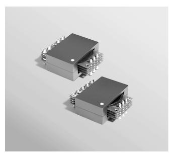
The PL140 surface mount planar transformers are rated for 140 Watts and are designed to operate between 200 kHz and 500 kHz. They are available in 15 turns ratios and six different schematics, and may be special ordered with an auxiliary winding.
