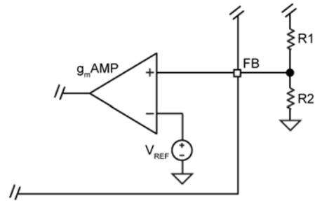
Figure 8. Voltage-Divider Configuration
