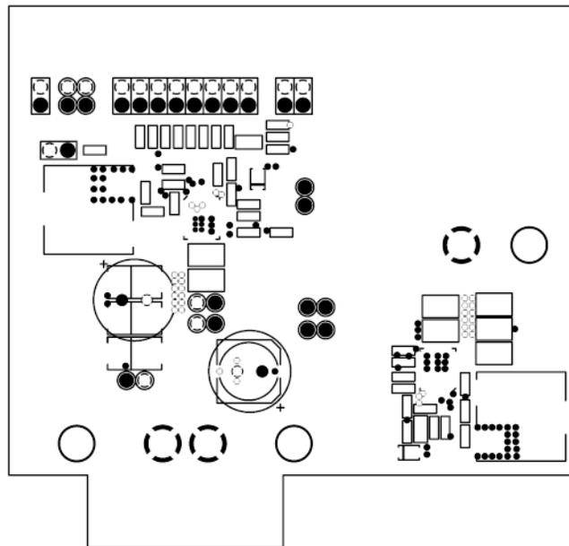
Figure 13. MIC24051 Evaluation Board Mid-Layer 1 (Ground Plane)
