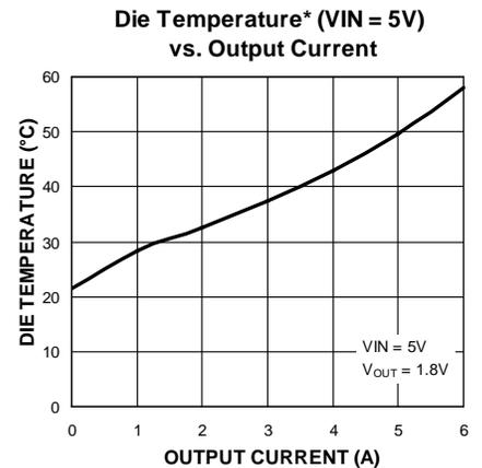
**Die Temperature\*** : The temperature measurement was taken at the hottest point on the MIC24051 case mounted on a 5 square inch 4 layer, 0.62", FR-4 PCB with 2oz finish copper weight per layer, see Thermal Measurement section. Actual results will depend upon the size of the PCB, ambient temperature and proximity to other heat emitting components.
