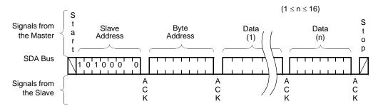
Figure 11. Writing 12 bytes to a 16-byte page starting at location 10.
