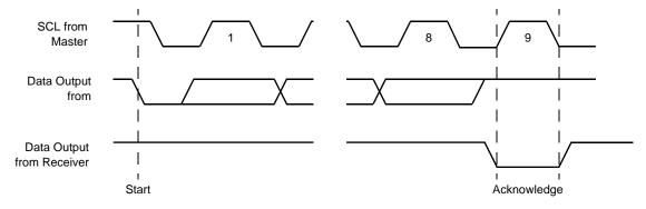
Figure 9. Byte Write Sequence
