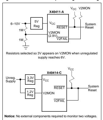
Figure 2. V<sub>TRIPX</sub> Set/Reset Conditions
