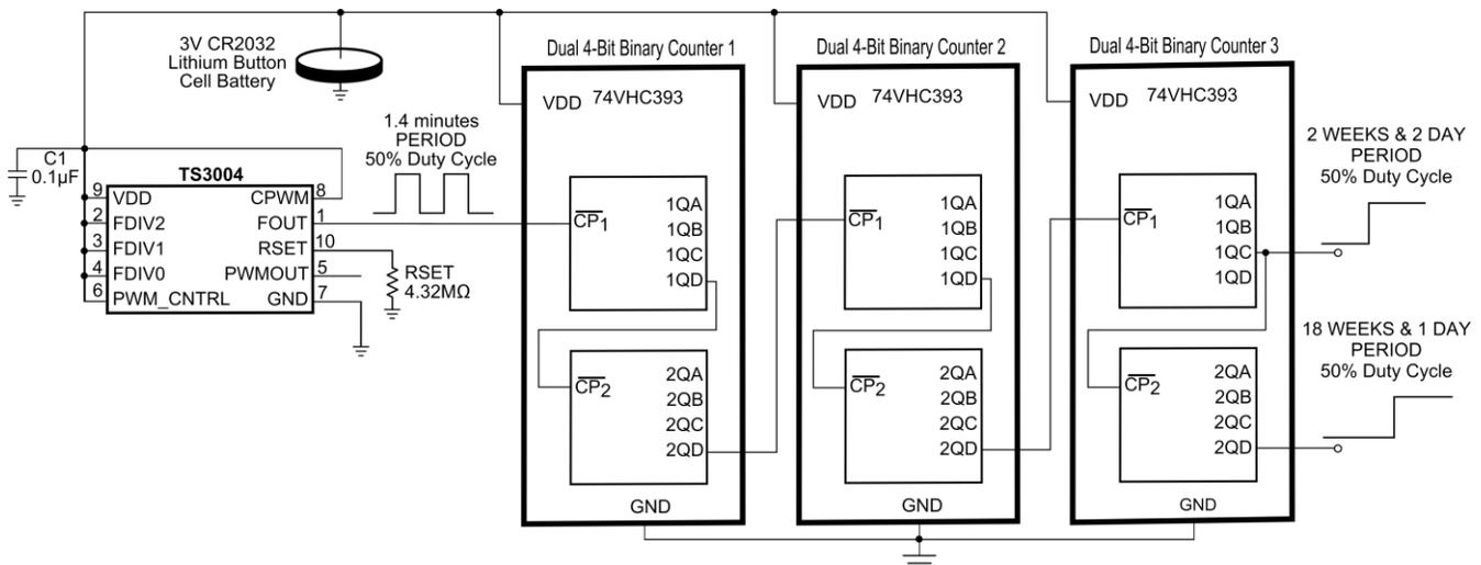
**Figure 2:** 2 Weeks and 2 Days Counter Circuit
