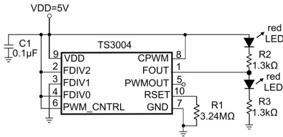
**Figure 4:** Flashing Railroad Lights with the TS3004
