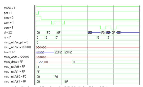
6.3 Setting and Reading the I/O Mode for P0 and P1
