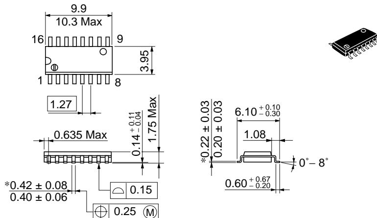
\*Dimension including the plating thickness
