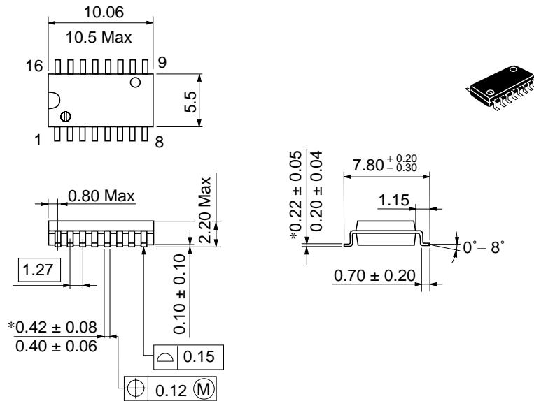
\*Dimension including the plating thickness
