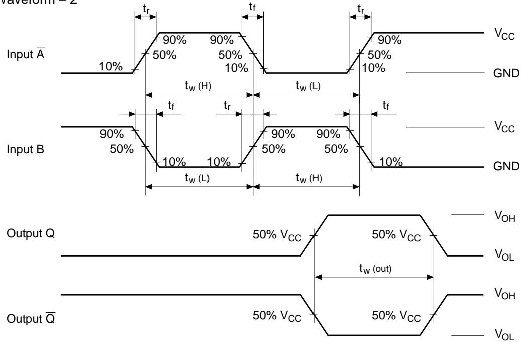
Notes: 1. Input waveform: PRR  $\leq$  1 MHz,  $Z_o = 50 \Omega$ ,  $t_r \leq 3$  ns,  $t_f \leq 3$  ns
