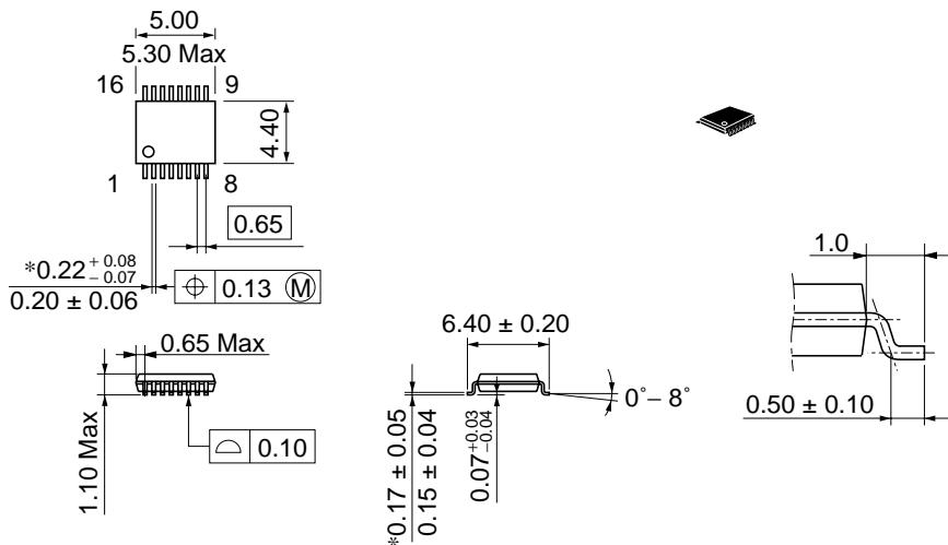
\*Dimension including the plating thickness
