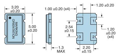
Note: Pin 1 Chamfer not shown.
