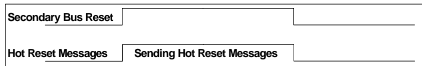
Figure 3-13. Secondary Bus Reset and Hot Reset Message Timing in Reverse Transparent Bridge Mode
