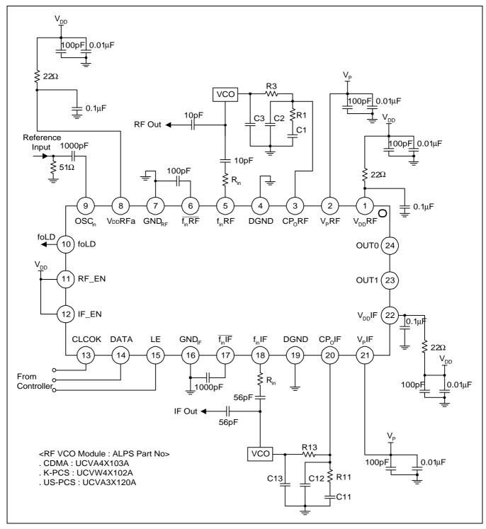
The role of Rin : Rin makes a large portion of VCO output power go to the load rather than the PLL. The value of Rin depends on the VCO power level
