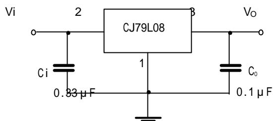
Note 1:Bypass capacitors are recommended for optimum stability and transient response and should be located as close as possible to the regulators.
