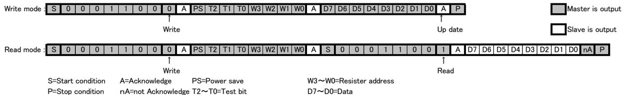
○ Characteristics of the SDA and SCL bus lines for 2-wire serial interface.
