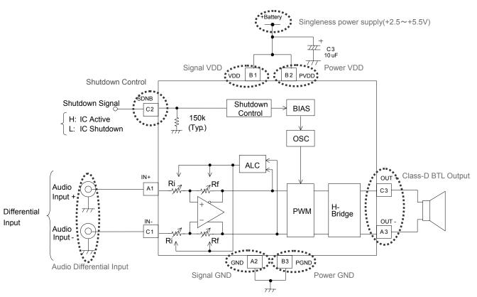
Fig2. Differential Input(Without Input Coupling Capacitor)
