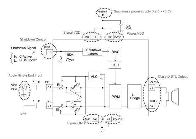
Fig3. Single end input (during IN+ input)
