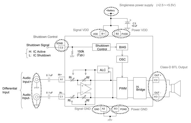
Fig1. Differential Input(With Input Coupling Capacitor)
