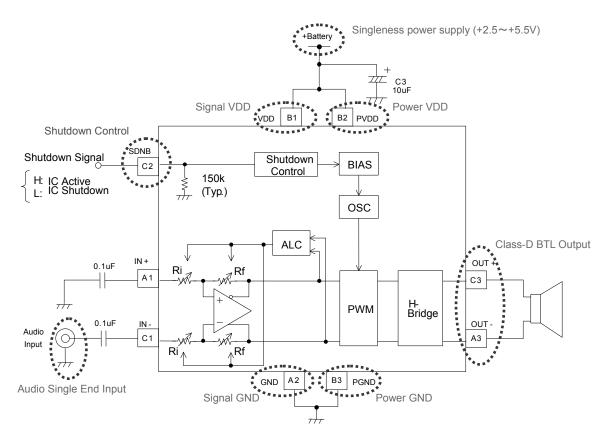
Fig4. Single end input (during IN- Input)
