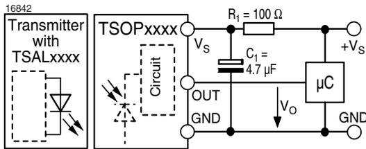
$R_1 + C_1$  recommended to suppress power supply disturbances.
