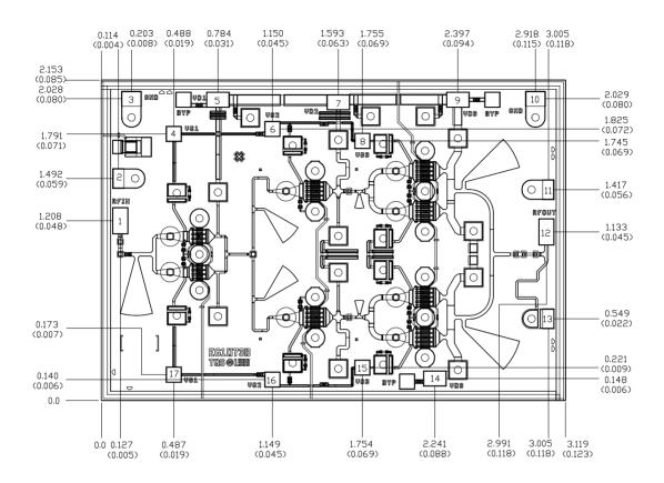
Units: millimeters (inches) Thickness: 0.1016 (0.004)
