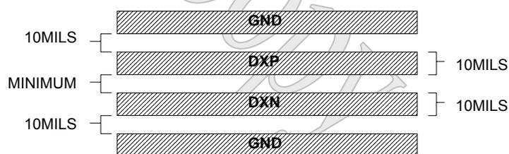
3. Use wide tracks to minimize inductance and reduce noise pickup. 10 mil track minimum width and spacing is recommended.
