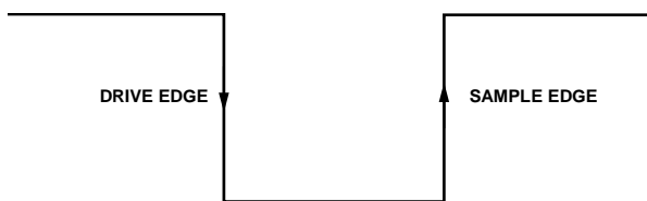
Figure 25. SPI Mode 3 SCLK Edges
