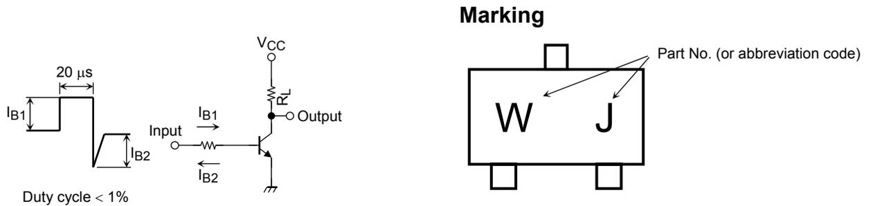
**Figure 1 Switching Time Test Circuit & Timing Chart**
