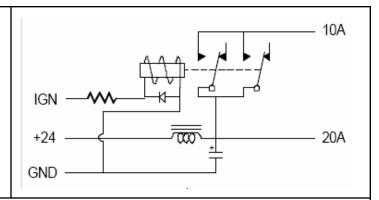
Operating voltage (max) = 12,24 or 36 Vdc Operating Current (max) = 20 Amperes Temperature range (storage) = -40 to 105 C Temperature range (operating) = -40 TO 65 C Design Specifications:
