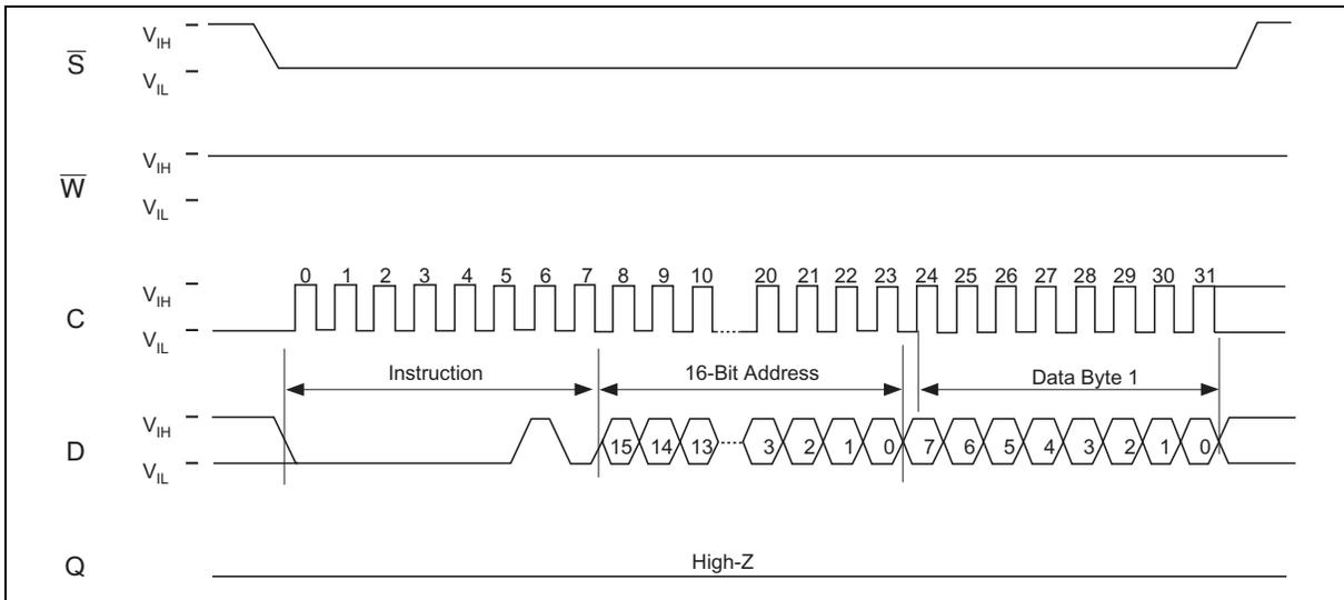
Note: 1. Depending on the memory size, as shown in Address Range Bits table, the most significant address bits are don't care.
