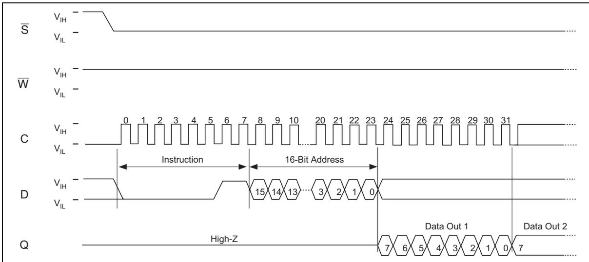
Note: 1. Depending on the memory size, as shown in the following table, the most significant address bits are don't care.
