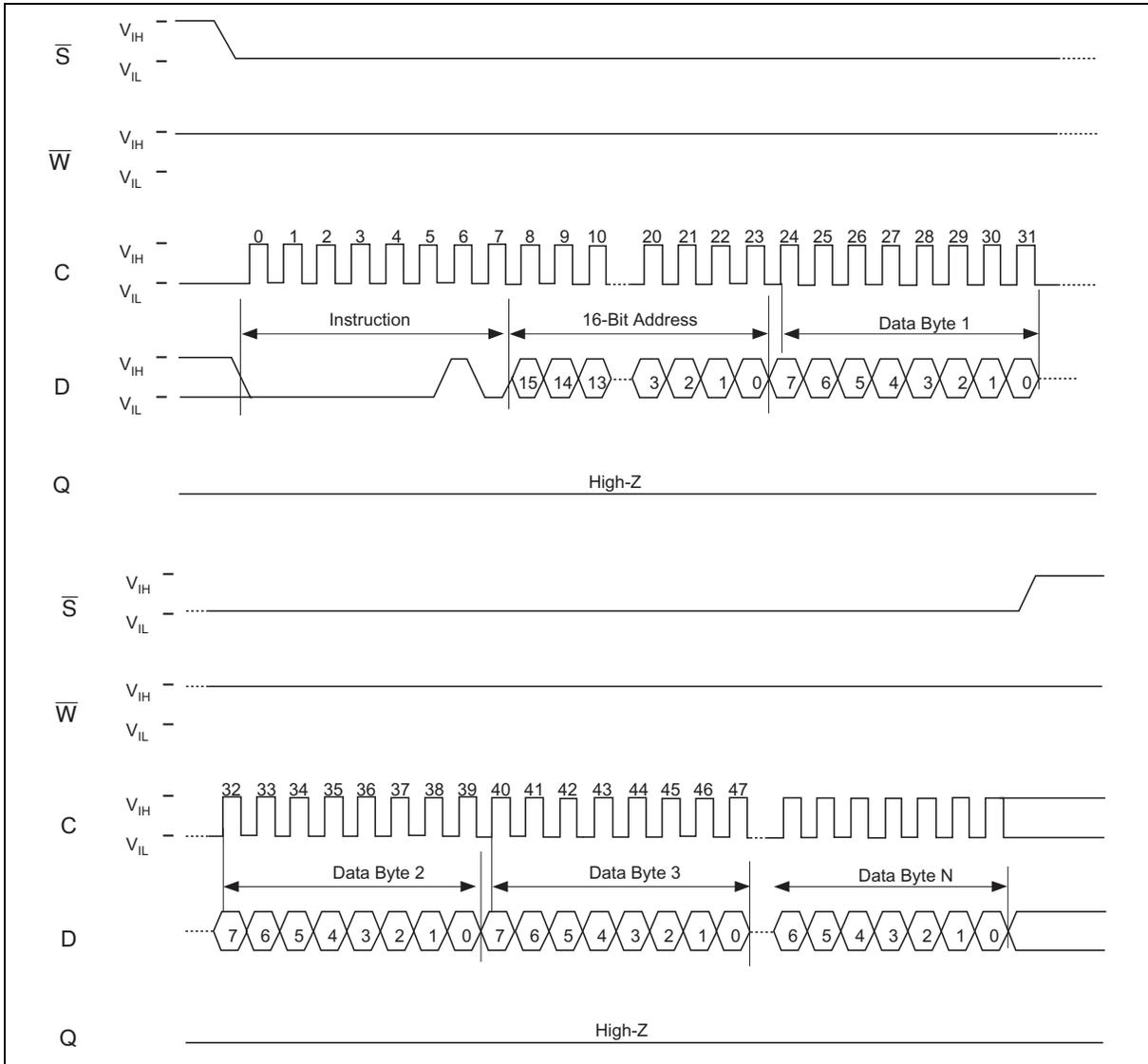
Note: 1. Depending on the memory size, as shown in Address Range Bits table, the most significant address bits are don't care.
