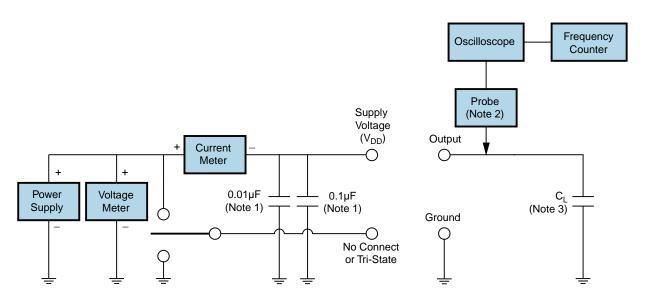
Note 1: An external  $0.1\mu\text{F}$  low frequency tantalum bypass capacitor in parallel with a  $0.01\mu\text{F}$  high frequency ceramic bypass capacitor close to the package ground and  $V_{DD}$  pin is required.
