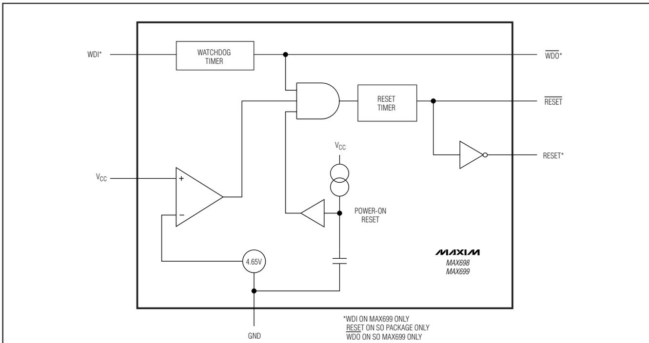
Figure 1. Block Diagram
