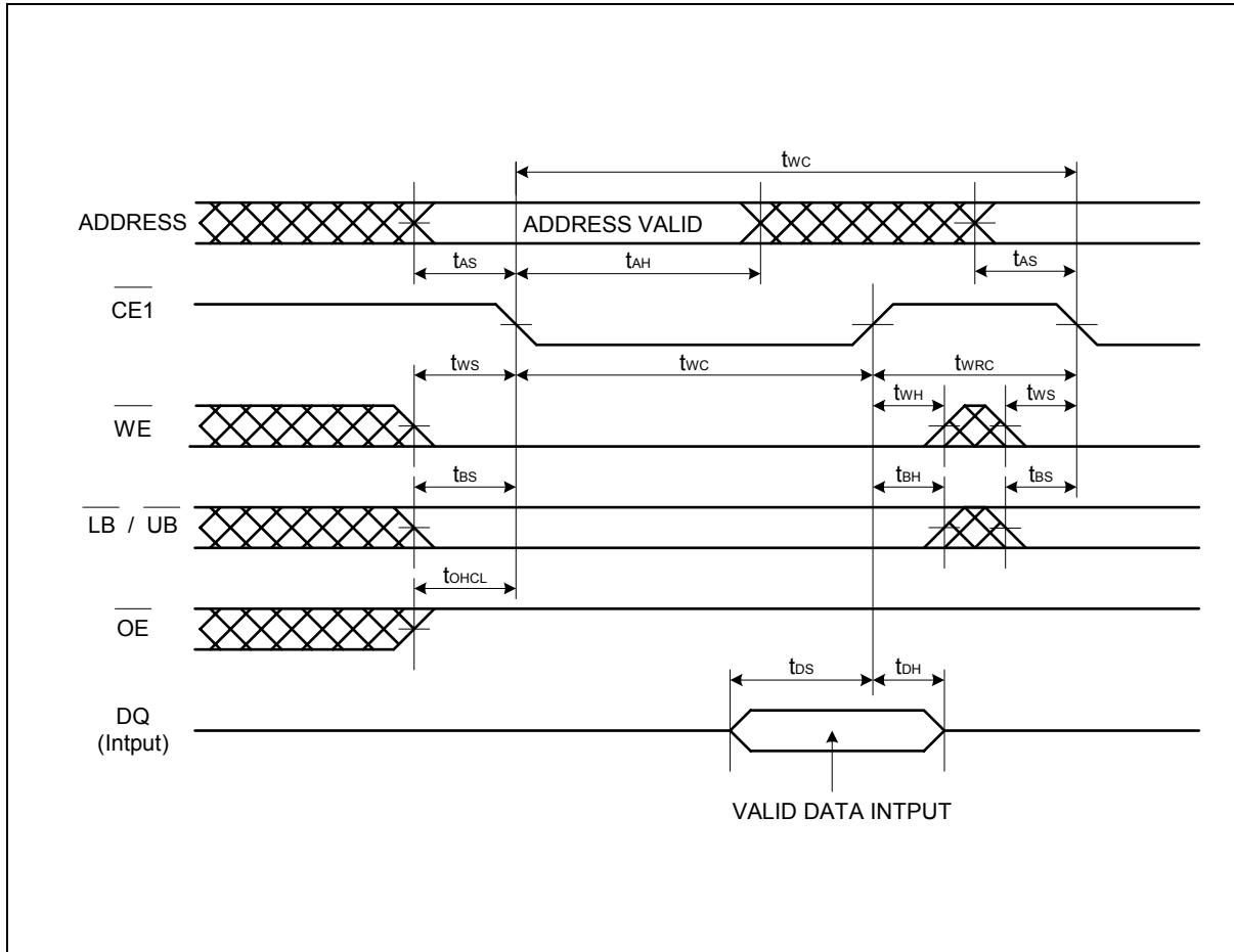
**Note:**  $\overline{CE2}$  and  $\overline{PE}$  must be High for entire write cycle.
