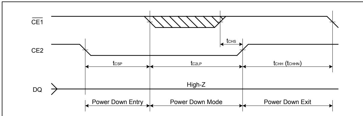
**Note:** This Power Down mode can be also used for Power-up #2 below except that  $t_{CHHN}$  can not be used at Power-up timing.
