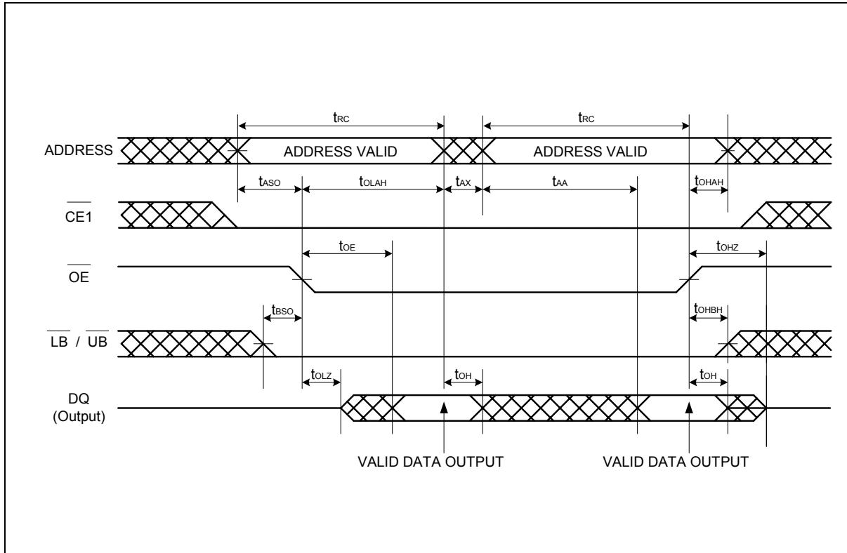
**Note:**  $\overline{CE2}$ ,  $\overline{PE}$  and  $\overline{WE}$  must be High for entire read cycle.
