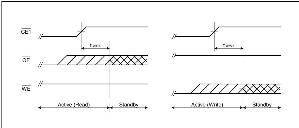
**Note:** Both  $t_{CHOX}$  and  $t_{CHWX}$  define the earliest entry timing for Standby mode. If either of timing is not satisfied, it takes  $t_{RC(\min)}$  period from either last address transition of A0, A1 and A2, or  $\overline{CE1}$  Low to High transition.
