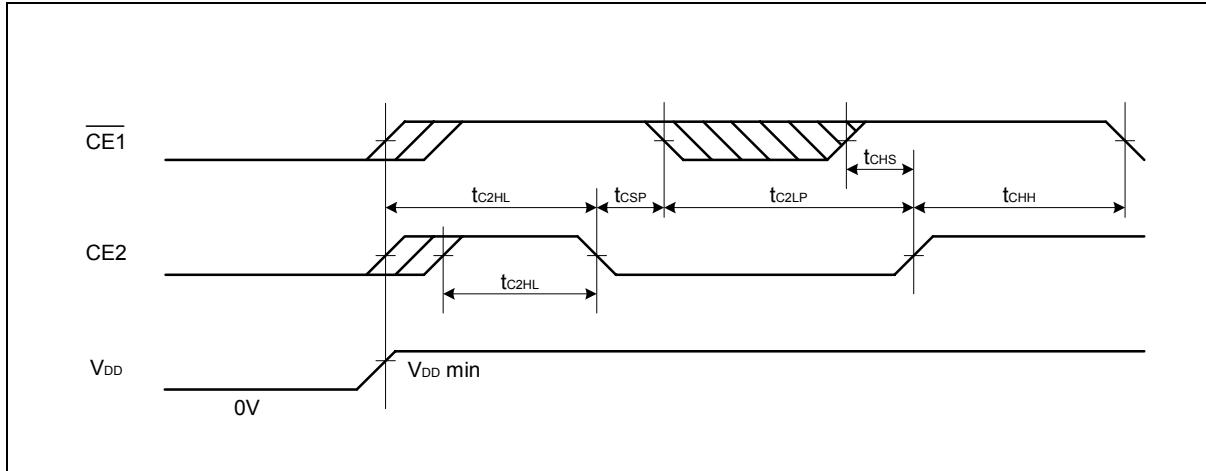
**Note:** The  $t_{C2HL}$  specifies from  $\overline{CE2}$  low to High transition after  $V_{DD}$  reaches specified minimum level.
