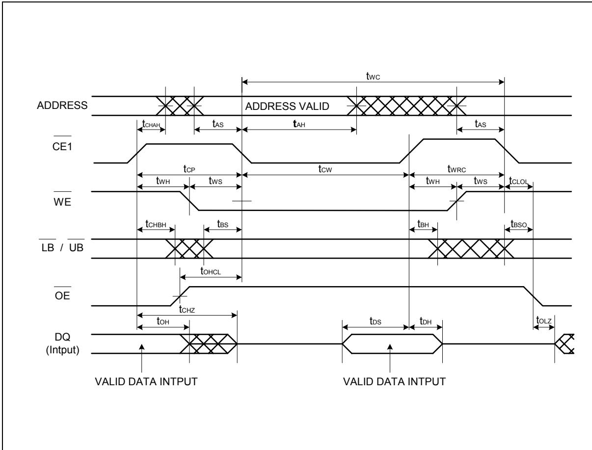
**Note:** Write address is valid from either  $\overline{CE1}$  or  $\overline{WE}$  of last falling edge.
