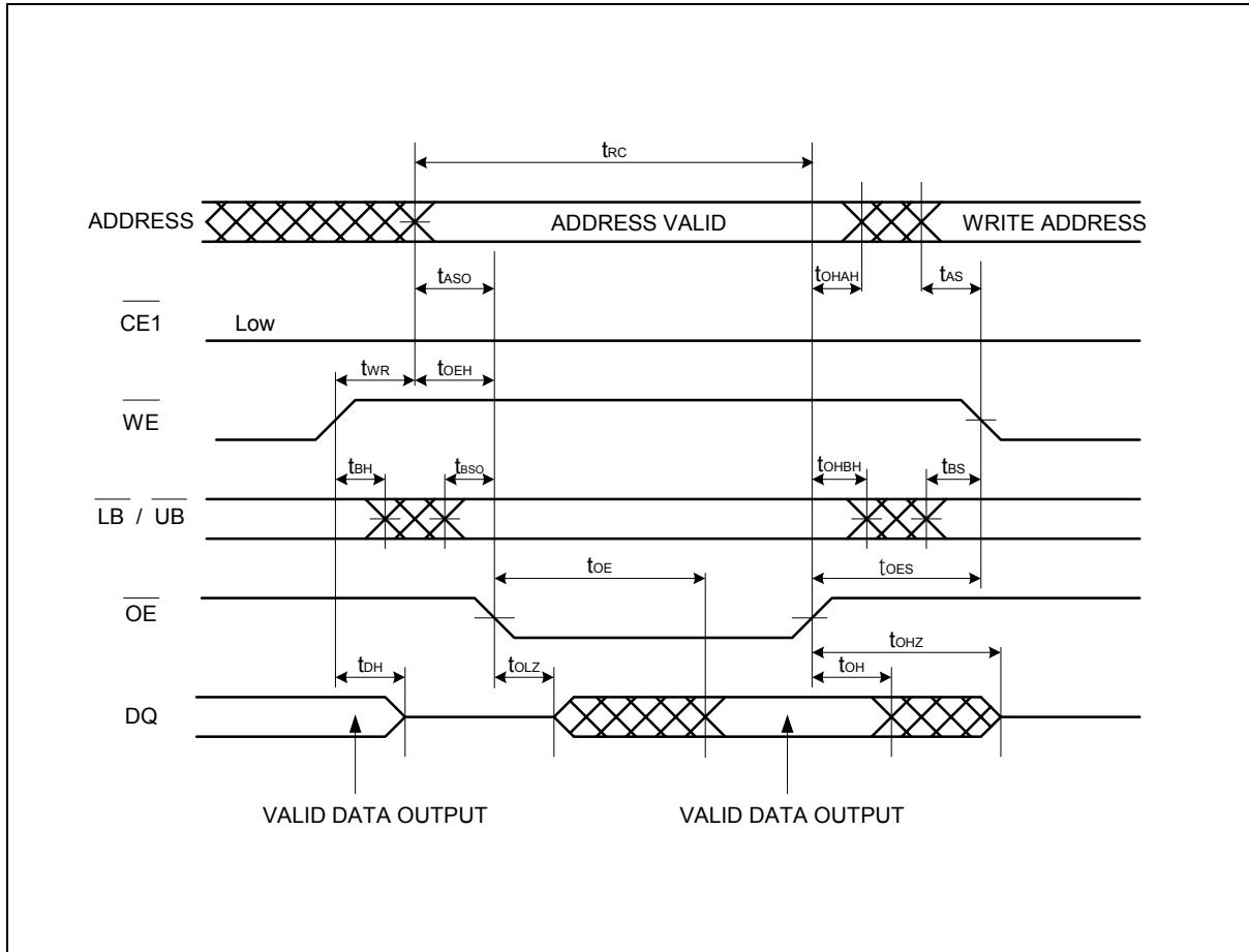
**Note:**  $\overline{CE1}$  can be tied to Low for  $\overline{WE}$  and  $\overline{OE}$  controlled operation.
