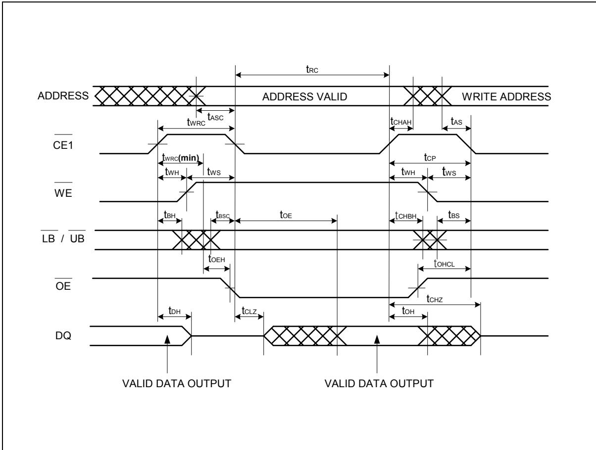
**Note:** The  $t_{OEH}$  is specified from the time satisfied both  $t_{WRC}$  and  $t_{WR(min)}$ .
