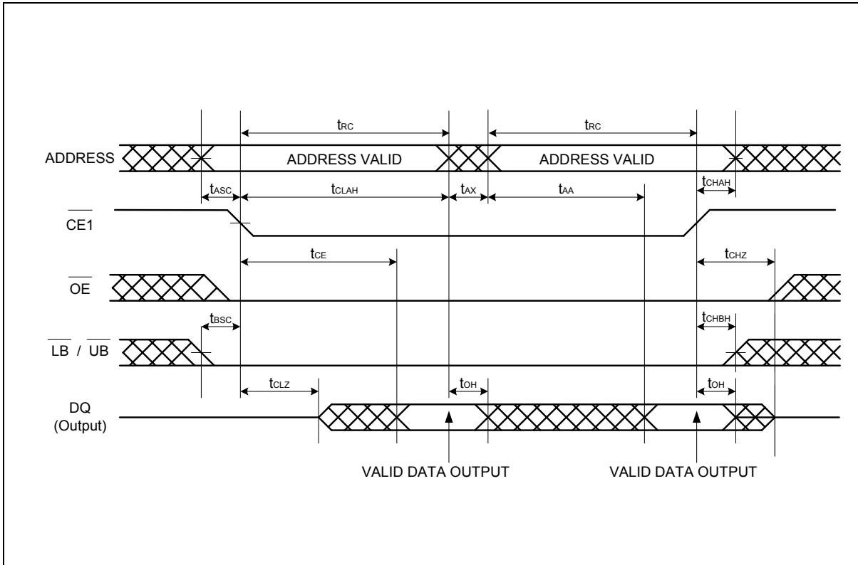
**Note:**  $\overline{CE2}$ ,  $\overline{PE}$  and  $\overline{WE}$  must be High for entire read cycle.
