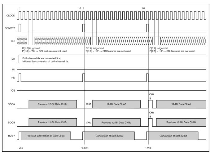
Figure 18. Mode III Timing Diagram (M0 = 1; M1 = 0)
