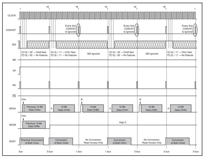
Figure 17. Mode II Timing Diagram (M0 = 0; M1 = 1)
