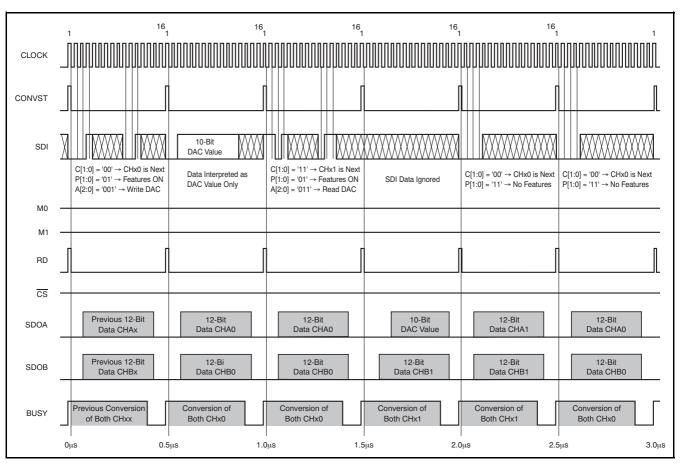
Figure 24. DAC Write and Read Access Timing Diagram
