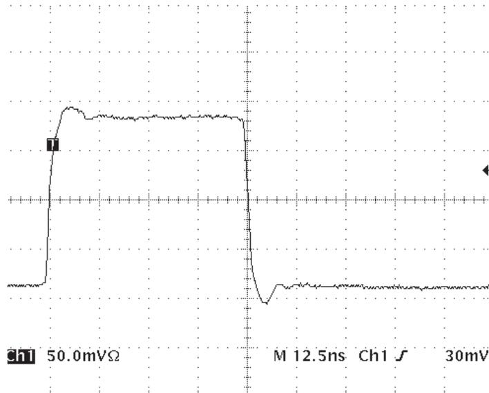
Figure 2: Pulse response, unity gain, 1V<sub>pp</sub>, R<sub>F</sub> = 510Ω
