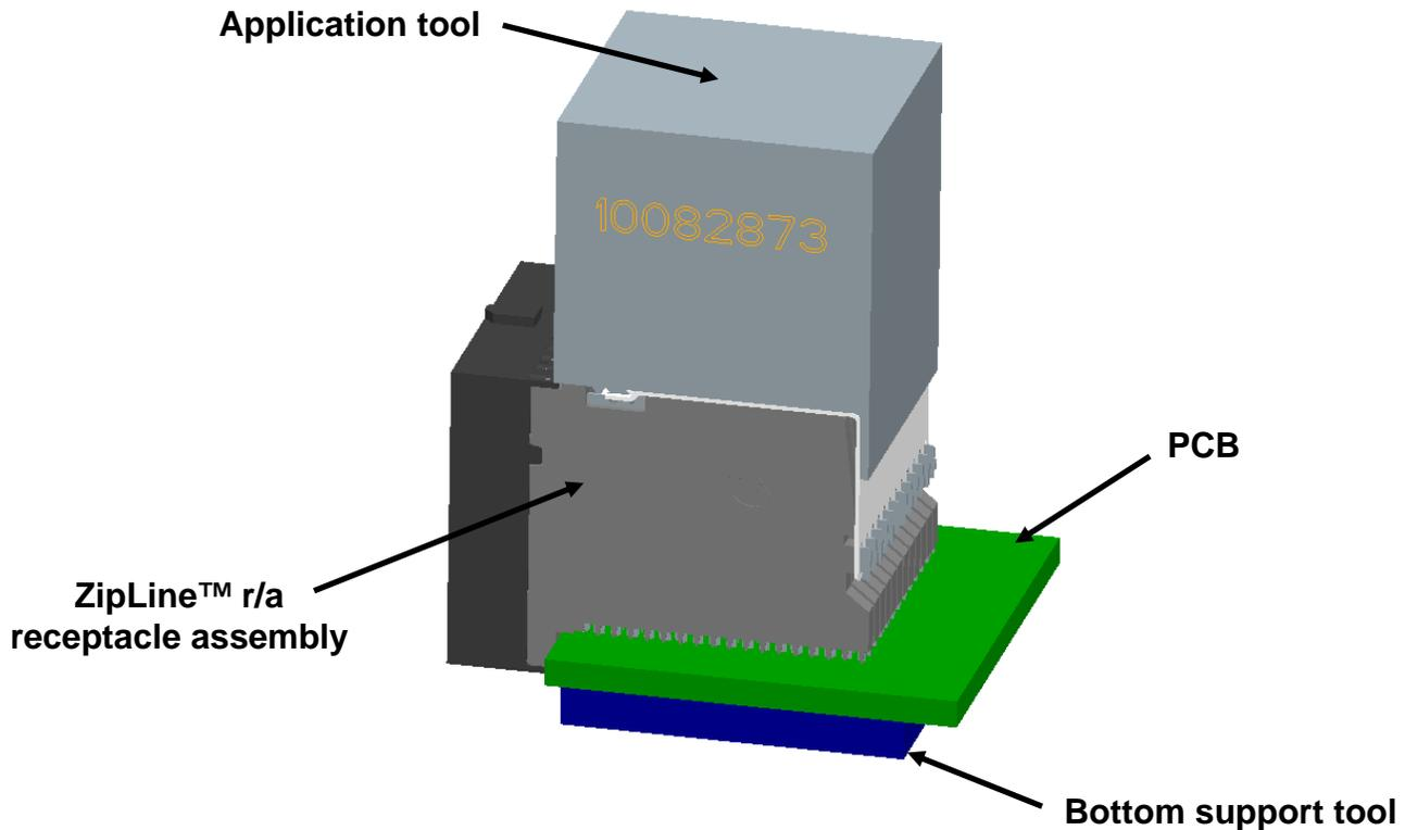
Figure 18: ZipLine™ right angle receptacle application tool (6pair, 12 IMLA shown)
