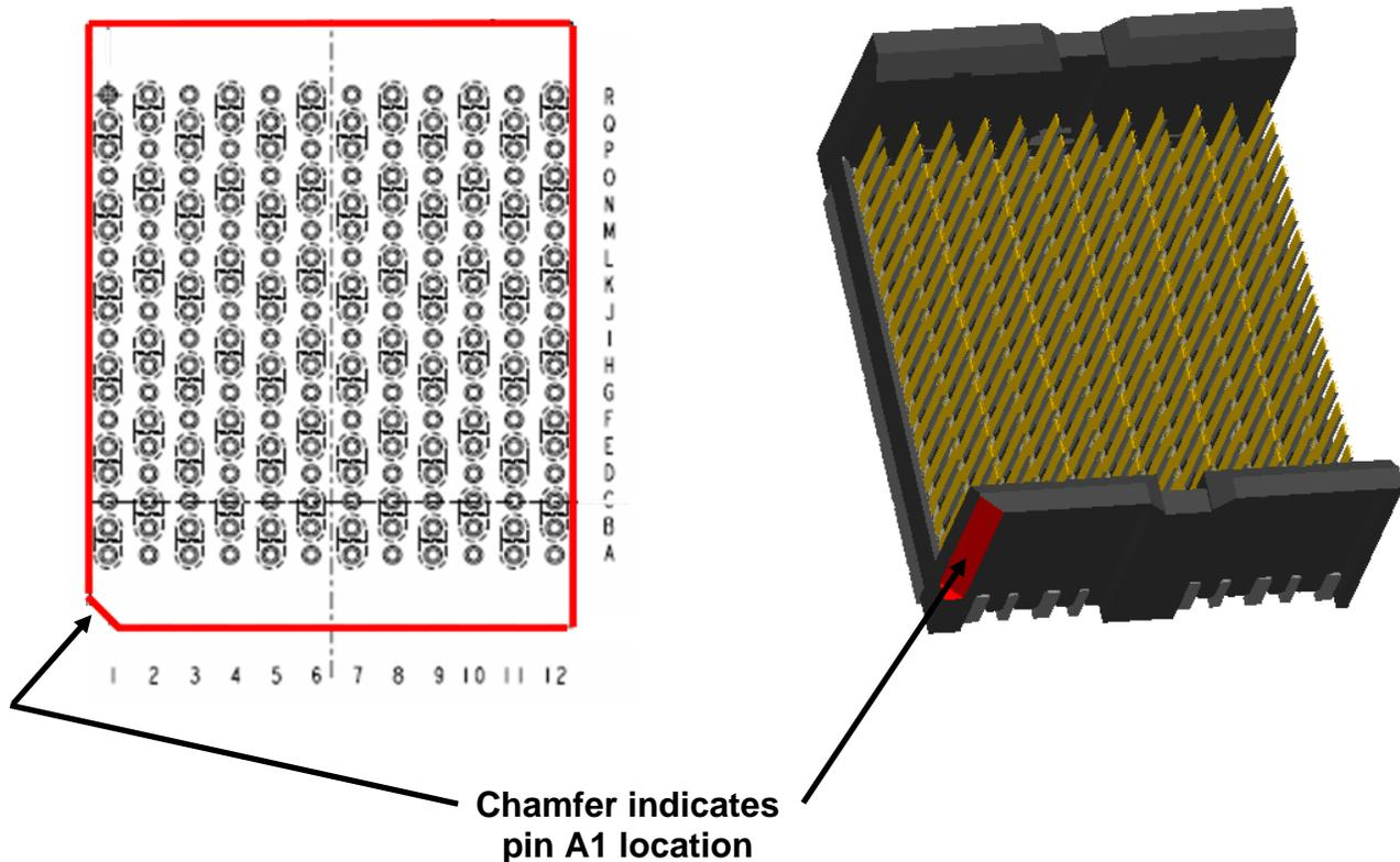
Figure 16: Vertical header outline with polarization feature
