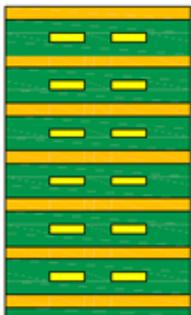
One differential pair per routing channel
