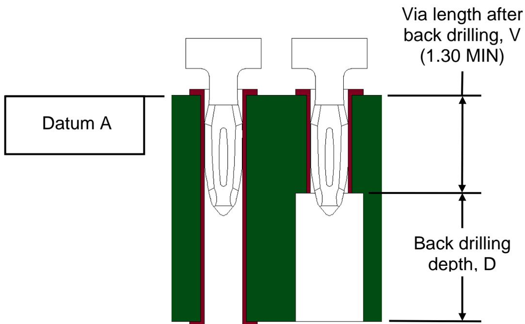
**Figure 15: Back drilled via's**
