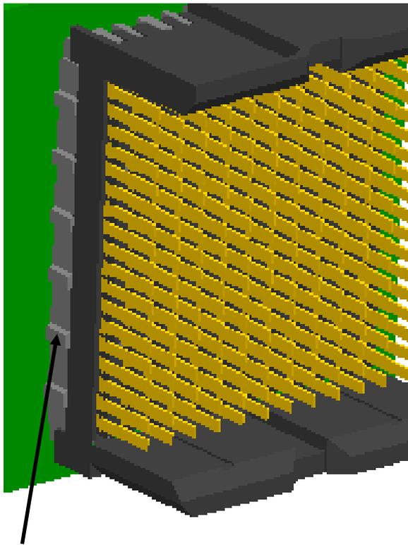
Protrusions are present on each side of an orthogonal header – must add 0.2mm extra space to avoid interference
