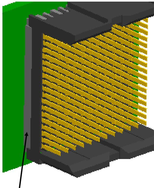
No protrusions are present on a standard backpanel header
