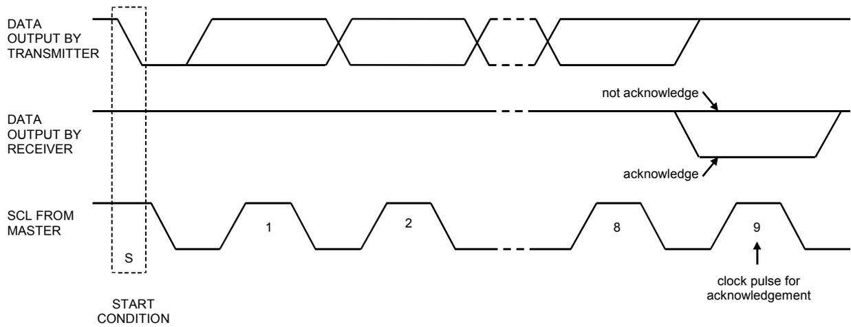
Figure 18. Acknowledge on the I<sup>2</sup>C-bus
