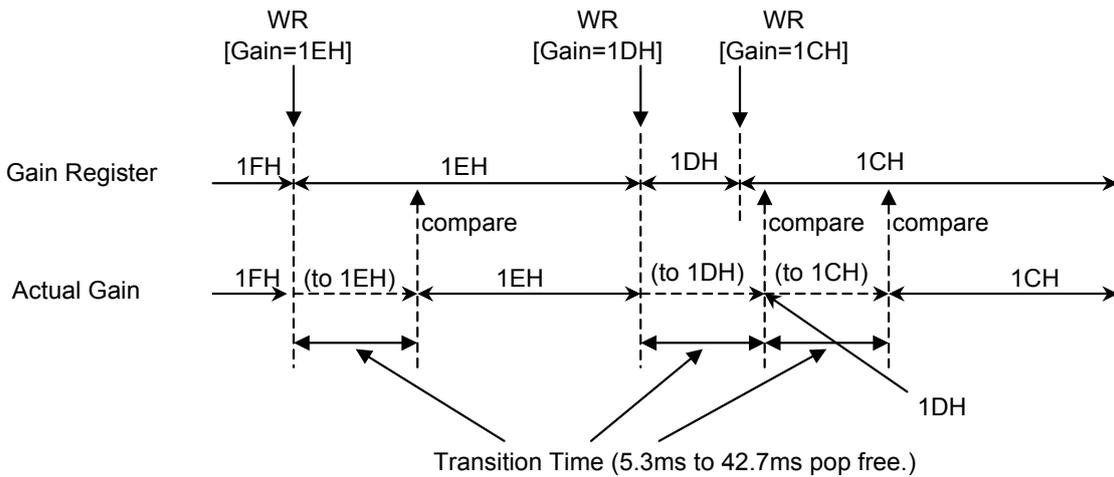
Figure 6. Volume Change Operation (MOD bit = "1")
