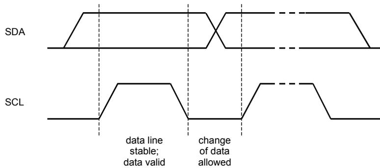
Figure 19. Bit transfer on the I<sup>2</sup>C-bus
