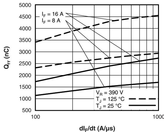
Fig. 10 - Typical Stored Charge vs.  $di_F/dt$
