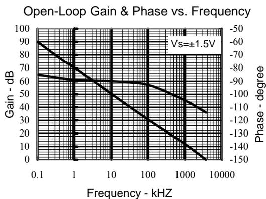
Test Condition:  $V_S = \pm 1.5\text{V}$ ,  $T_A = 25^\circ\text{C}$
