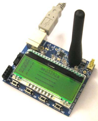
Figure 2. Si4313 LCD FSK/OOK Receiver Any-Band (P/N 4313-DACB ANY) with 434 MHz Antenna (P/N MSC-AT50-434)
