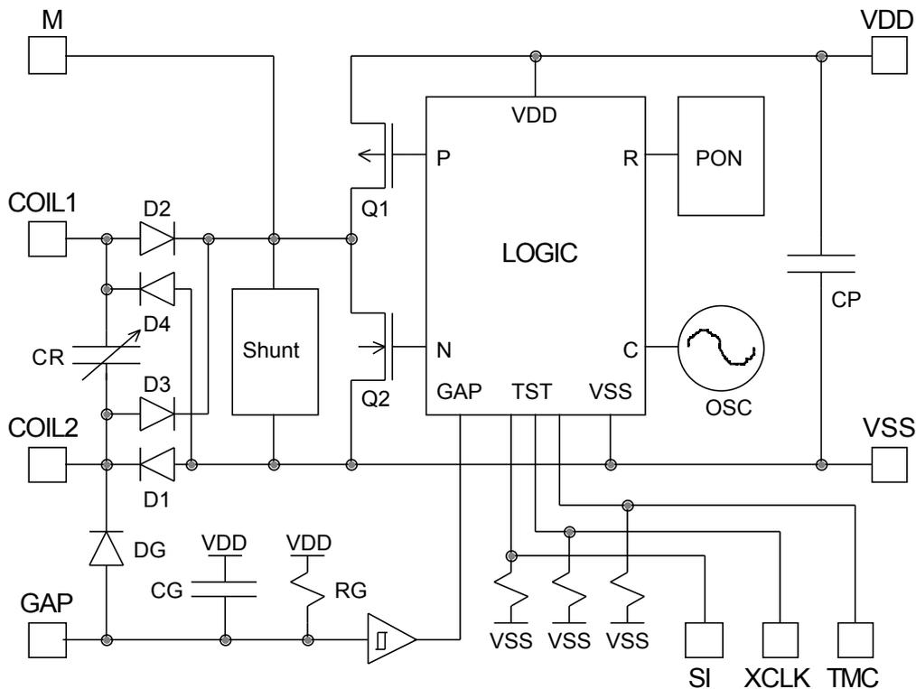
**Figure 4: P4022 Block diagram**
