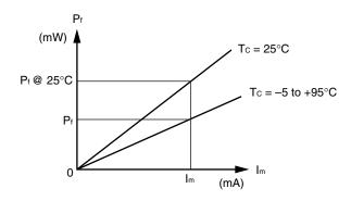
$$\gamma = \left| 10 \log \frac{P_f}{P_f @ 25^{\circ}C} \right| [dB]$$
