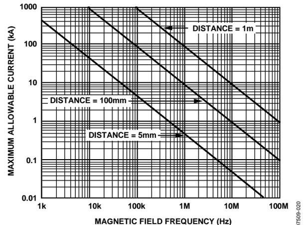
Figure 16. Maximum Allowable Current for Various Current-to-ADuM5400 Spacings
