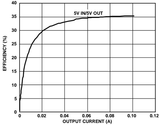
Figure 4. Typical Power Supply Efficiency at 5 V/5 V
