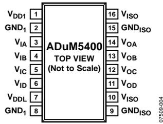
Figure 3. Pin Configuration
