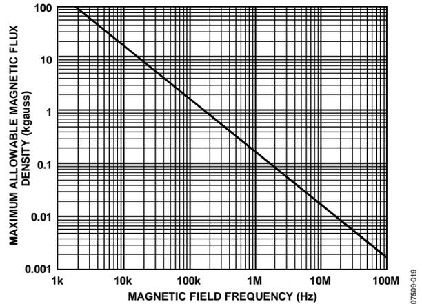
Figure 15. Maximum Allowable External Magnetic Flux Density
