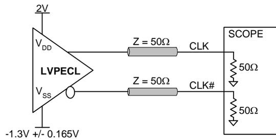
**Figure 3. 2.5V Output Load AC Test Circuit**
