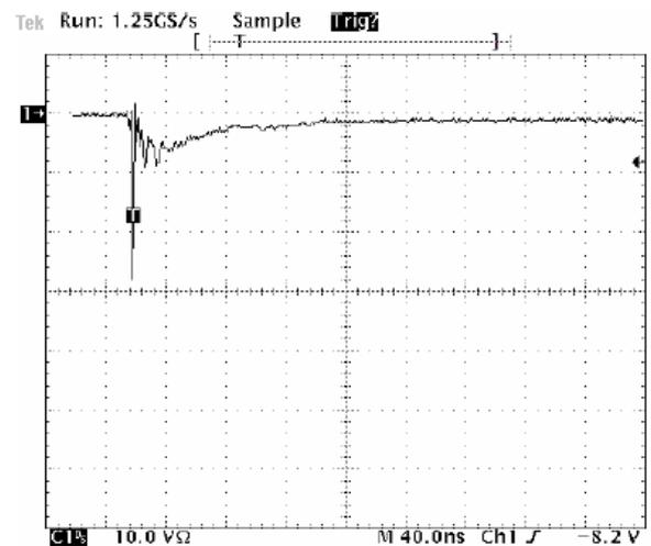
**Figure 5. Negative 8kV contact per IEC 61000-4-2-LESD7D5.0T5G**
