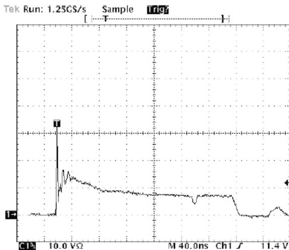
**Figure 4. Positive 8kV contact per IEC 61000-4-2-LESD7D5.0T5G**
