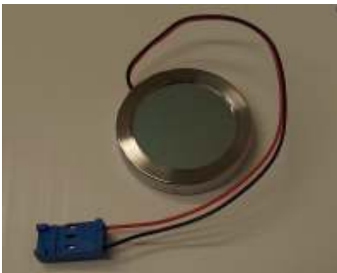
MSD024 detector supplied as an alpha monitor.
