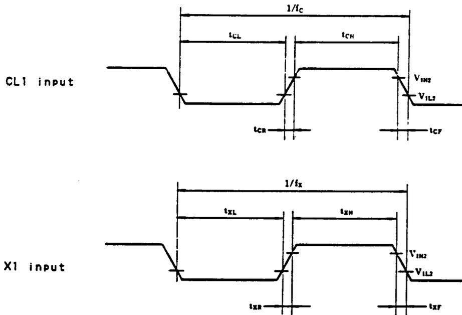
(a)  $2.7 \text{ V} \leq V_{DD} \leq 6.0 \text{ V} : V_{IH2} = V_{DD} - 0.5 \text{ V}, V_{IL2} = 0.5 \text{ V}$
