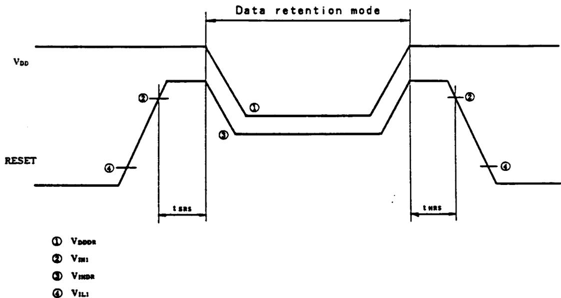
Caution: In the data retention mode, all inputs must be on  $V_{DDDR}$  or lower.
