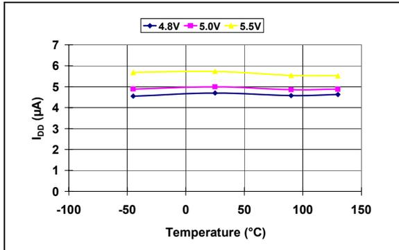
**FIGURE 2-7:**  $I_{DD}$  vs. Temperature (Watchdog Timer Active) (**MCP1318M-4.6**).
