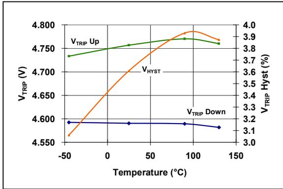
**FIGURE 2-16:**  $V_{TRIP}$  and  $V_{HYST}$  vs. Temperature (MCP1318M-4.6).
