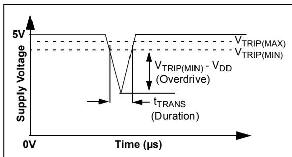
**FIGURE 4-16:** Example of Typical Transient Duration Waveform.
