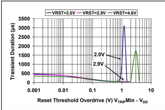
**FIGURE 2-34:** Transient Duration vs.  $V_{TRIP}(\text{min}) - V_{DD}$ .
