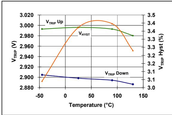
**FIGURE 2-17:**  $V_{TRIP}$  and  $V_{HYST}$  vs. Temperature (MCP1319-2.9).
