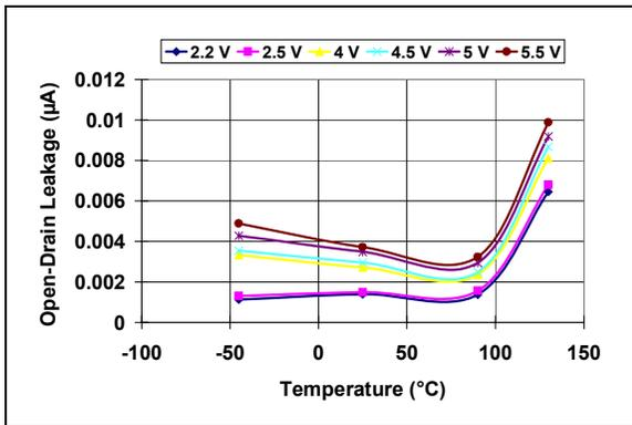
**FIGURE 2-35:** Open-Drain Leakage Current vs. Temperature (MCP1320-2.0).
