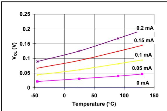
**FIGURE 2-23:**  $V_{OL}$  vs. Temperature (MCP1319-2.9 @  $V_{DD} = 2.7V$ ).
