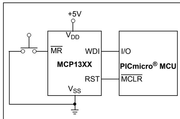
**FIGURE 4-17:** Push Button Reset and Watchdog Timer.
