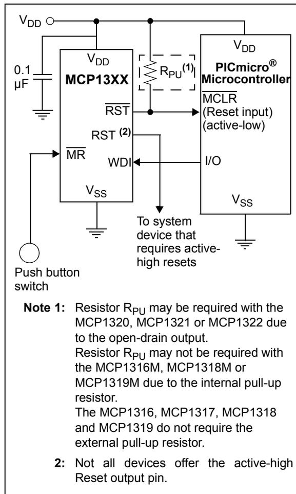
FIGURE 4-1: Typical Application Circuit.
