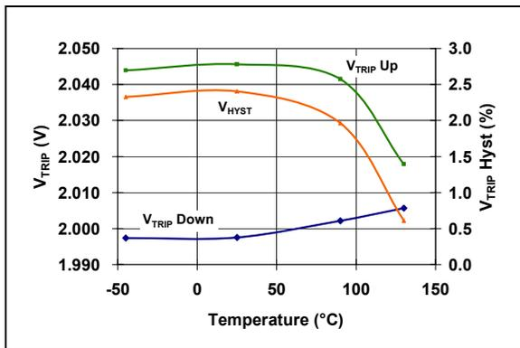
**FIGURE 2-18:**  $V_{TRIP}$  and  $V_{HYST}$  vs. Temperature (MCP1316-2.0).
