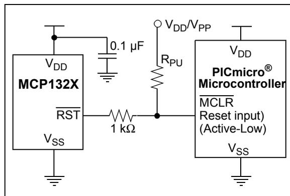
**FIGURE 5-4:** Typical Application Circuit for PICmicro<sup>®</sup> Microcontroller with the ICSP<sup>™</sup> Feature.
