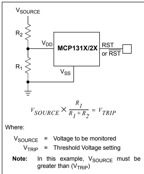
**FIGURE 5-5:** Modify Trip-Point using External Resistor Divider.
