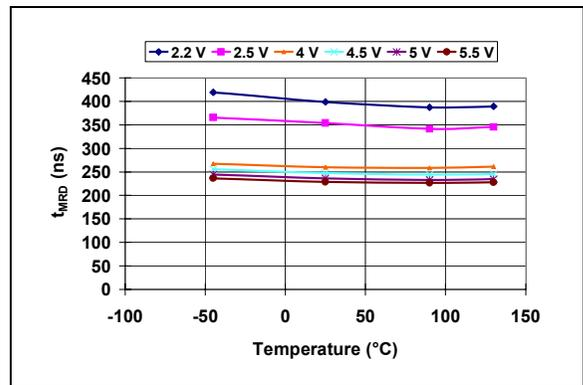
**FIGURE 2-38:**  $\overline{\text{MR}}$  Low to Reset Propagation Delay (MCP1316-2.0).
