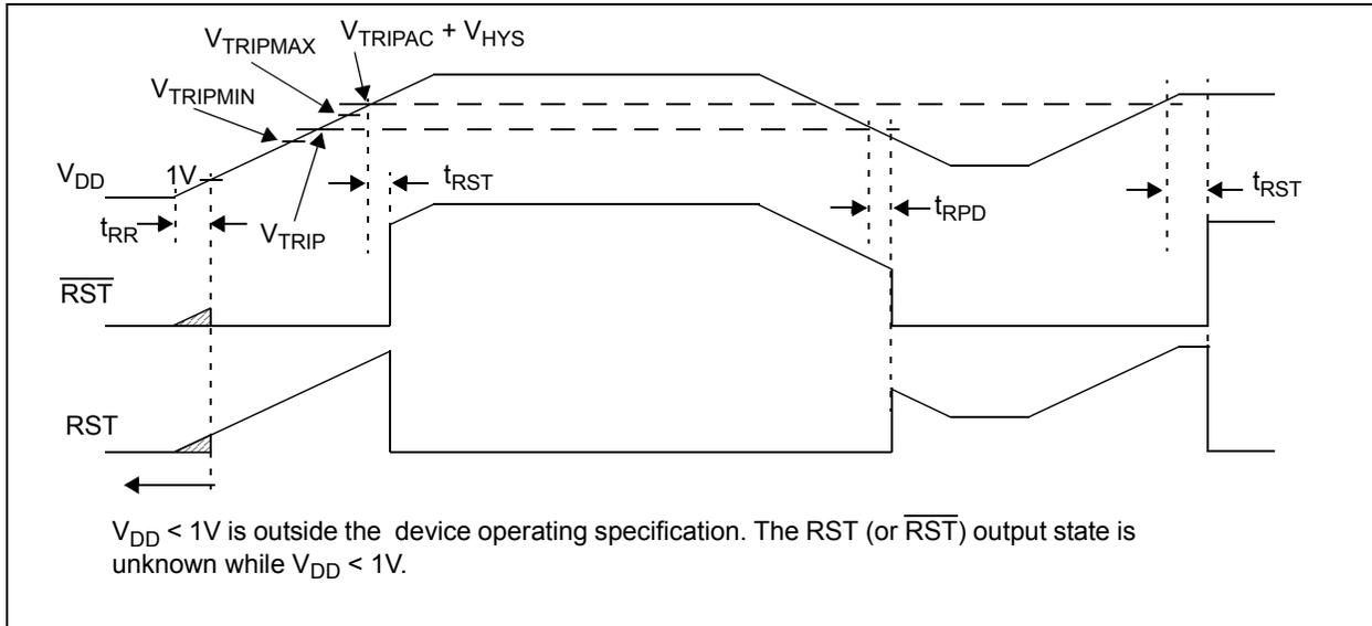
**FIGURE 1-1:** Device Voltage and Reset Pin Waveforms.
