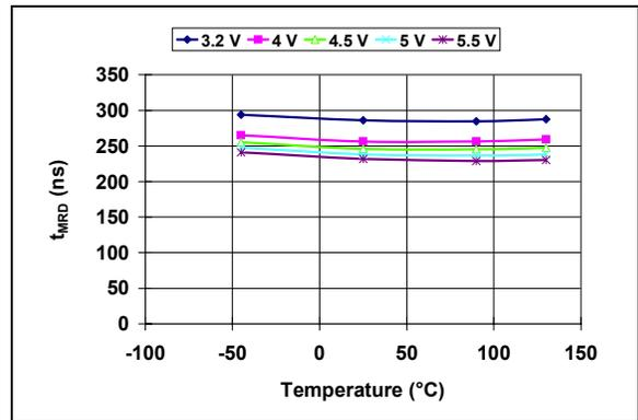
**FIGURE 2-37:**  $\overline{\text{MR}}$  Low to Reset Propagation Delay (MCP1319-2.9).
