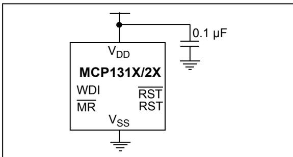
**FIGURE 5-1:** Typical Application Circuit with Bypass Capacitor.
