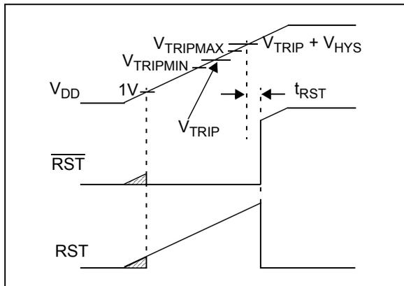
**FIGURE 4-13:** Reset pin Operation on a Power-up.
