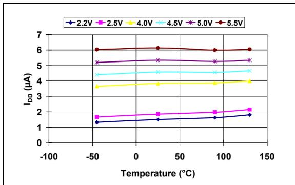
**FIGURE 2-9:**  $I_{DD}$  vs. Temperature (Watchdog Timer Active) (**MCP1316-2.0**).
