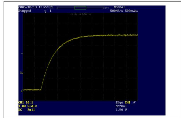
**FIGURE 2-49:** "M" Part # Pull-up Characteristics (MCP1318M-4.6).
