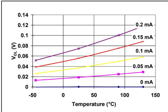
**FIGURE 2-22:**  $V_{OL}$  vs. Temperature (MCP1318M-4.6 @  $V_{DD} = 4.5V$ ).
