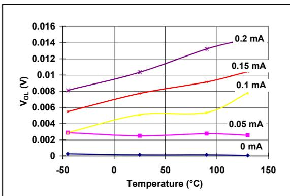
**FIGURE 2-24:**  $V_{OL}$  vs. Temperature (MCP1316-2.0 @  $V_{DD} = 1.8V$ ).
